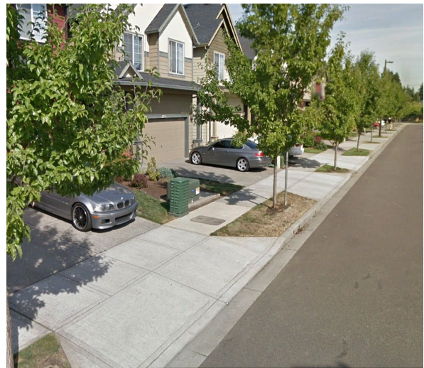
Allowing driveways to occupy more of the property frontage potentially impacts the pedestrian environment and reduces on-street parking.
