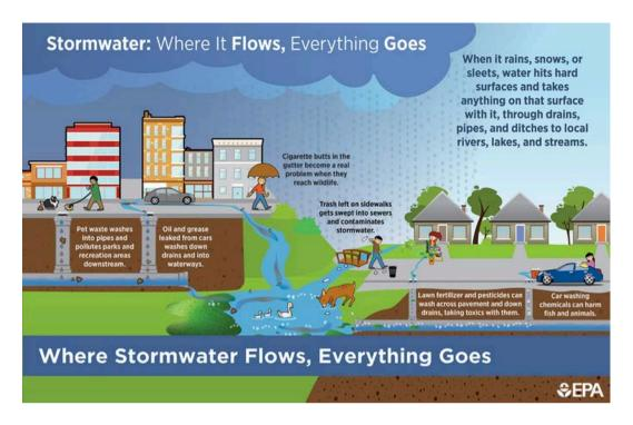
Anything that enters a storm sewer system (i.e. a drain, catch basin, ditch, etc.) is eventually discharged untreated into the bodies of water we use for swimming, fishing, and irrigation.
