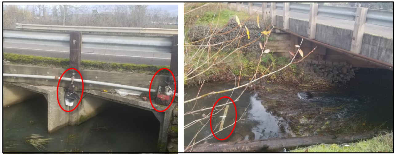
Figure 2-7. Left: Depth Meter Installed on Monmouth Cutoff Road (NF Tributary); Right: Flow Meter Installed on Godsey Road (NF Ash Creek)
